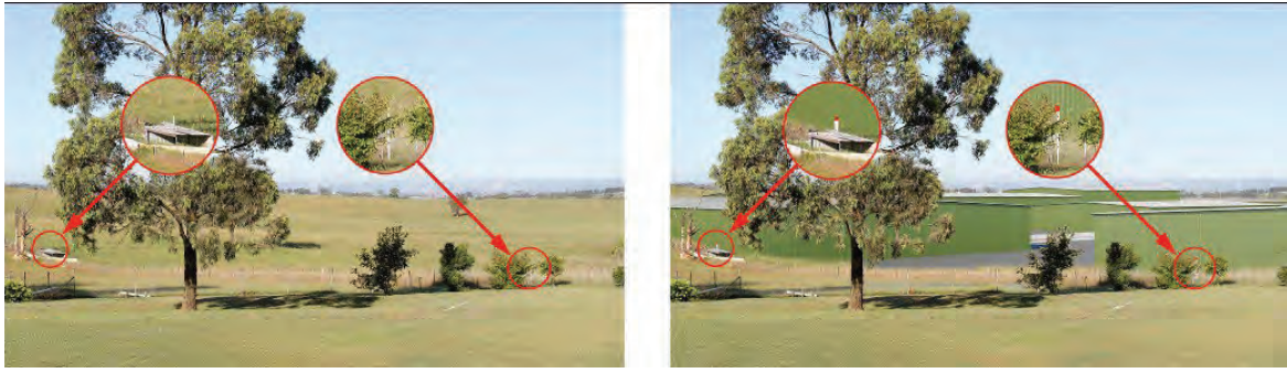
Physical 3000mm site poles placed at lot corners 3d poles located in the 3d model and positioned on photo
