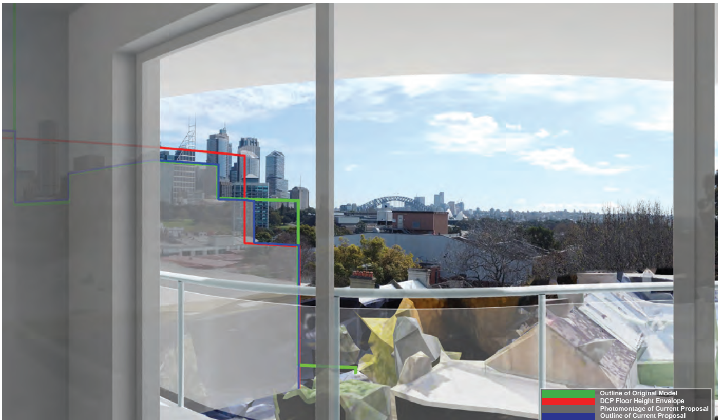
Viewpoint 38: Photomontaged virtual view, showing permitted building height envelope and new proposal.
